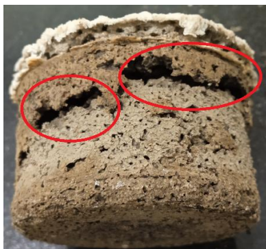
Sample C5 at 180°C : S42.86; Water content 55.65%; %NaCl: 42.86%;
