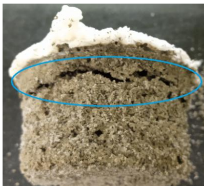
Sample C2 at 120°C : S38.82; Water content 51.04%; %NaCl: 38.82%;
