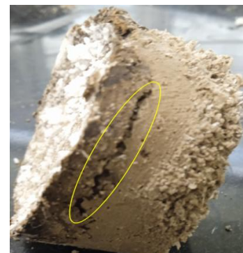
Sample C2 at 90°C : S24.71; Water content 78.81%; %NaCl: 41.28%;
