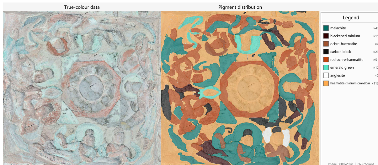
Fig. 8 Wall-scale hyperspectral inversion example. Left: true-colour composite. Right: per-pixel pigment classification map. Library spectra were resampled to the camera bands (400–1000 nm) and pixels classified by weighted matching ( w = 0.5 ) with re-calibrated graded rejection thresholds, leaving sub-threshold pixels unclassified; the legend gives the per-class counts of spatially contiguous same-class regions (263 in total).
