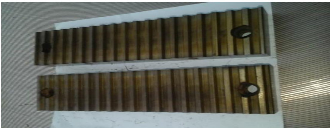
Figure 2.3 Honeycomb core die
