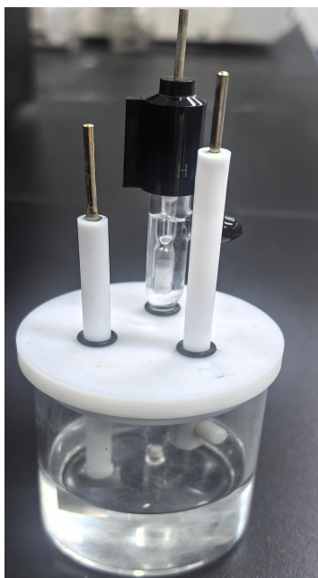
Fig. S8. Digital photograph of the three-electrode electrolyzer.
