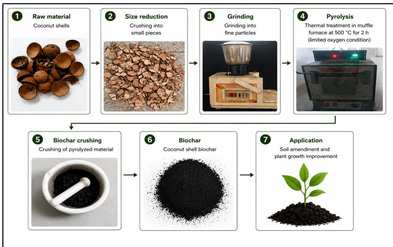
Fig. 1 Process flow of synthesize of biochar from coconut shell waste
