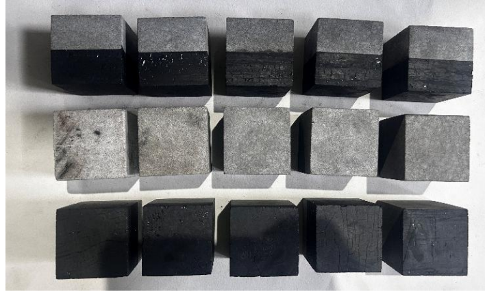
Fig. 1 The tested rock specimens with different lithologies
