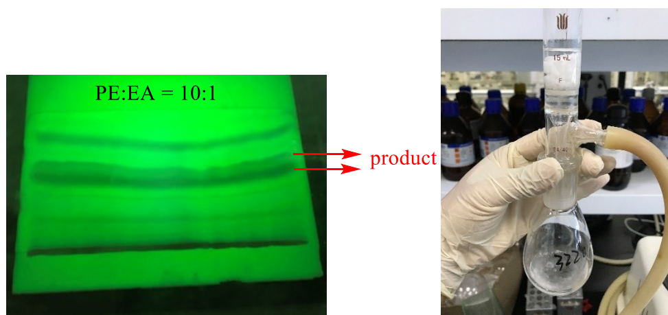
Fig. S6 Step 6: Purified by preparative thin-layer chromatography (PTLC) (eluent: petroleum ether:ethyl acetate = 10:1), note that both bands should be collected.
