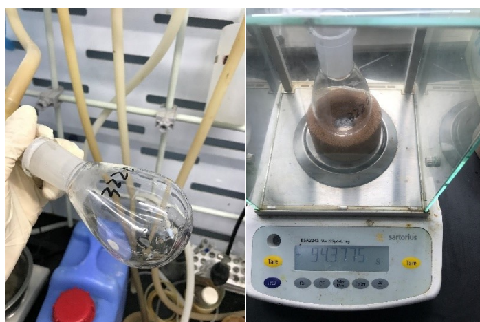
Fig. S7 Weight of product (55.5 mg, 74% yield). Pure product is a colorless oil.
