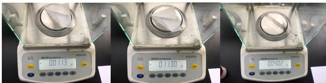
Fig. S3 Step 3: TAC + (11.3 mg, 0.024 mmol), Et 4 NBF 4 (113.0 mg, 0.52 mmol, 0.1 M), n -butylbenzene (40.2 mg, 0.3 mmol), added to the cell.
