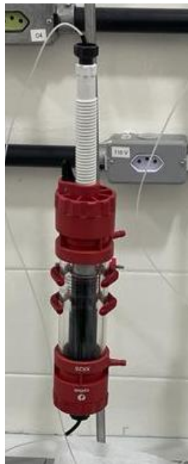
Figure 1. Column containing only biochar for the passage of the saline solution for washing.
