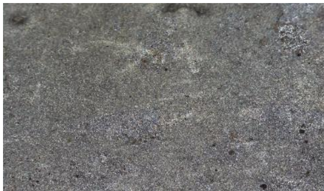
Figure 6. Optical Microscopic image of austenitic 316L stainless steel after immersion in 9 M HCl solution. (mag x 10).
