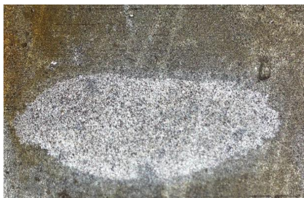
Figure 7. Optical Microscopic image of austenitic 316L stainless steel after immersion in 9 M HCl solution and SI. (mag x 10).
