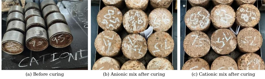
Fig. 4 Compacted specimens (a) before curing, and after curing at 40 °C for three days for (b) the anionic-stabilized mix and (c) the cationic-stabilized mix
