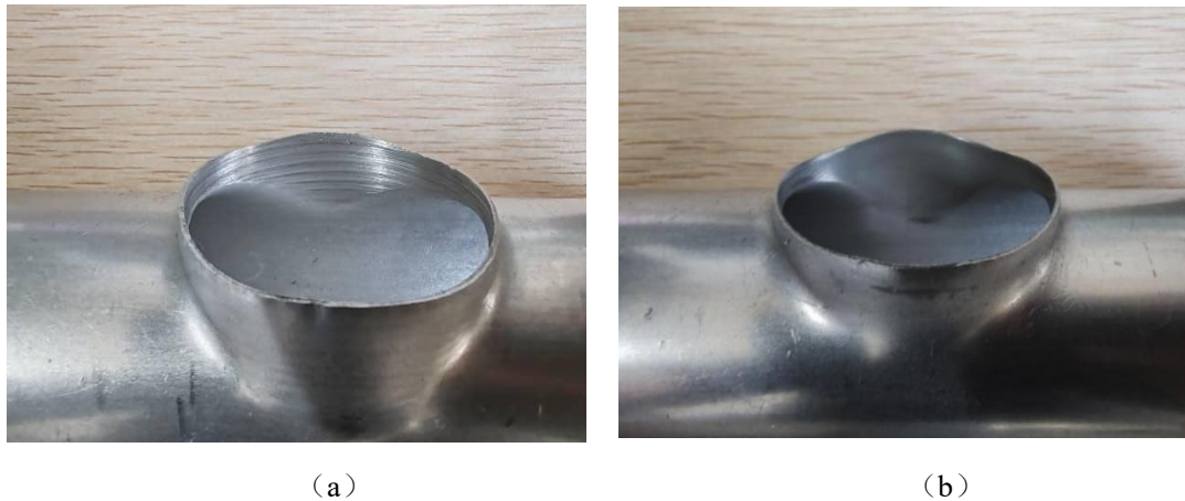
Fig. 11 Surface topography of branch pipes after two types of rotary head forming (a) Integral rotary head (b) Ball-type rotary head
