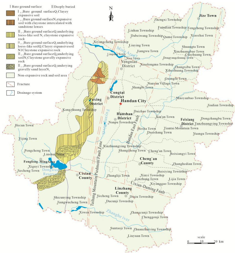
Fig. 1 Distribution of expansive soils (rocks) along the Handan section of the Middle Route of the South-to-North Water Diversion Project
