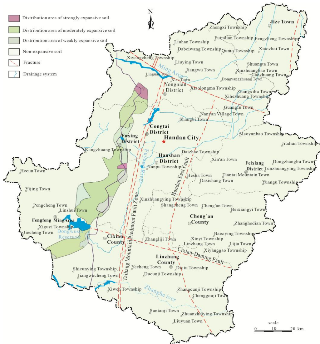
Fig. 2 Distribution of expansive soils (rocks) of different swelling grades along the Handan section of the Middle Route of the South-to-North Water Diversion Project
