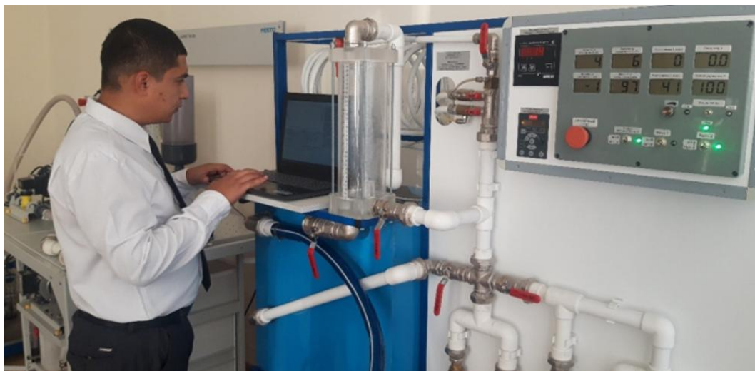
Figure 9. Experimental work on the upgraded laboratory test bench “Centrifugal Pumps” SGU-TsNS-012-6LR-PK.
