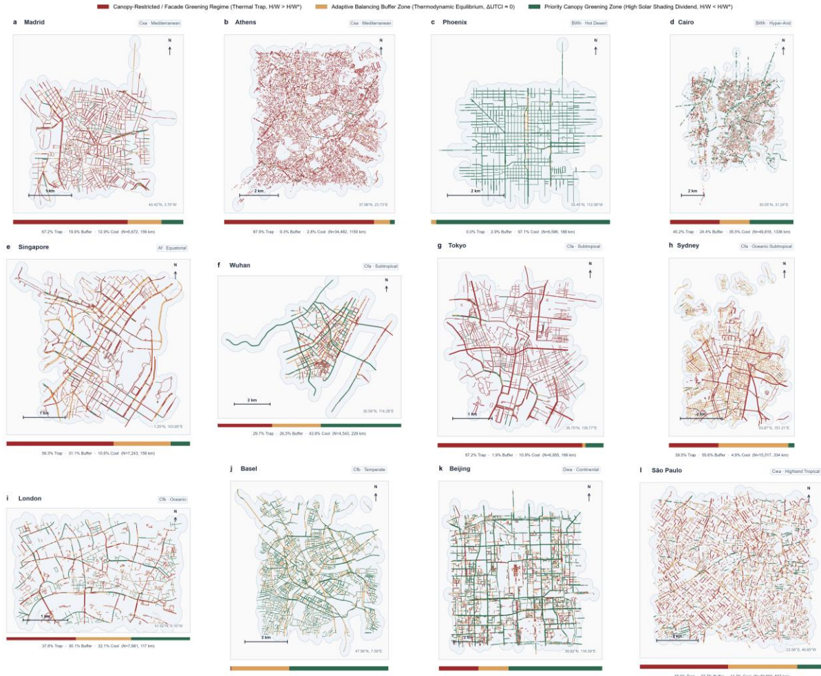
Figure 2 | Global geospatial bifurcation of street canyon microclimate regimes across 12 megacities. Length-weighted spatial distribution of nocturnal thermal liabilities (aerodynamic-radiative trapping, crimson), neutral thermodynamic equilibrium (amber), and priority canopy greening / net daytime cooling (forest green) under an intensive 30% street canopy benchmark ( f_{tree} = 0.30 ). Subpanels display high-density morphological core networks mapped with built-up urban fabric footprints and road hierarchy across Madrid, Athens, Phoenix, Cairo, Singapore, Wuhan, Tokyo, Sydney, London, Basel, Beijing, and São Paulo (204,267 authentic corridors, 5,898 km). Top headers display Köppen climate classifications and segment counts; bottom indicator bars show empirical percentage shares and total street length.
