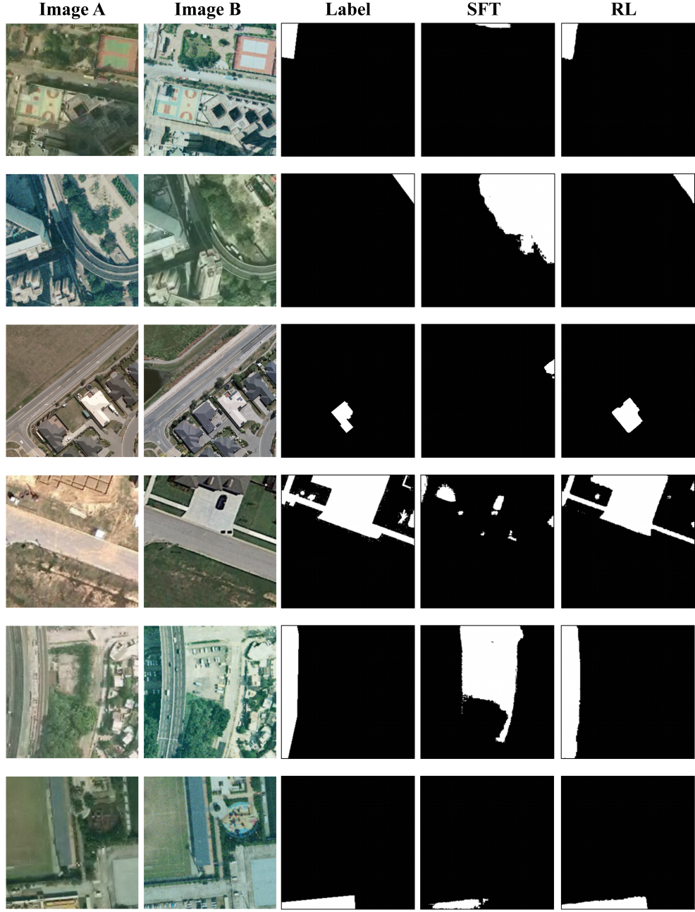
Fig. 8: Qualitative comparison on change detection. Since Falcon weights are not publicly available, we compare VectorLLM++ before and after RL post-training; RL improves change-mask completeness and changed-object localization.
