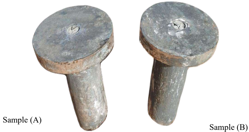
Fig. 3. As-cast ASTM A216 steel specimens prepared for the comparative evaluation of the reference and Ti-modified conditions.
