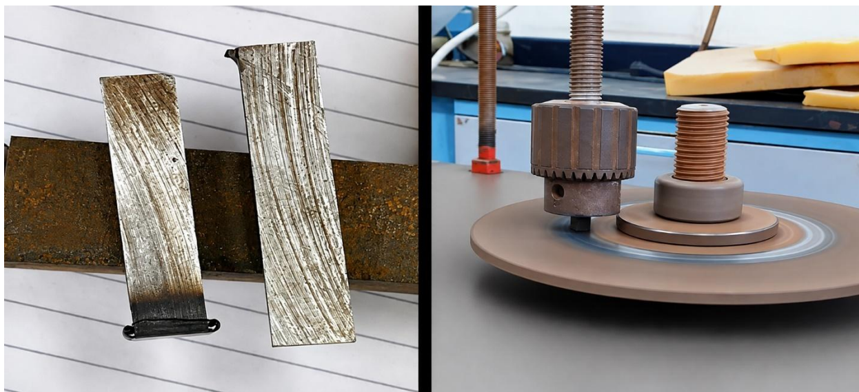
Fig. 11. Macroscopic appearance of the worn surfaces of the reference and Ti-modified ASTM A216 cast-steel specimens after pin-on-disk testing.
