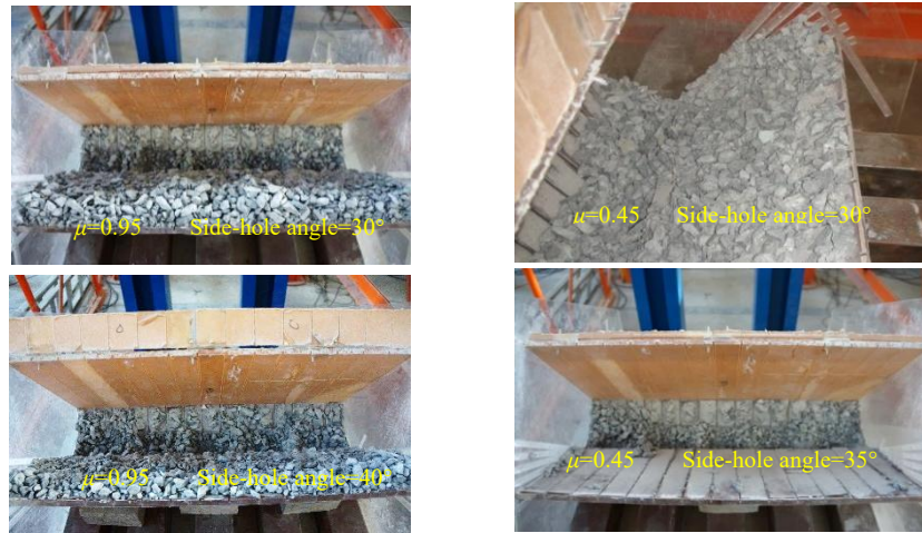
(a) Ore residuals at different side-hole angles under ore fragment friction
