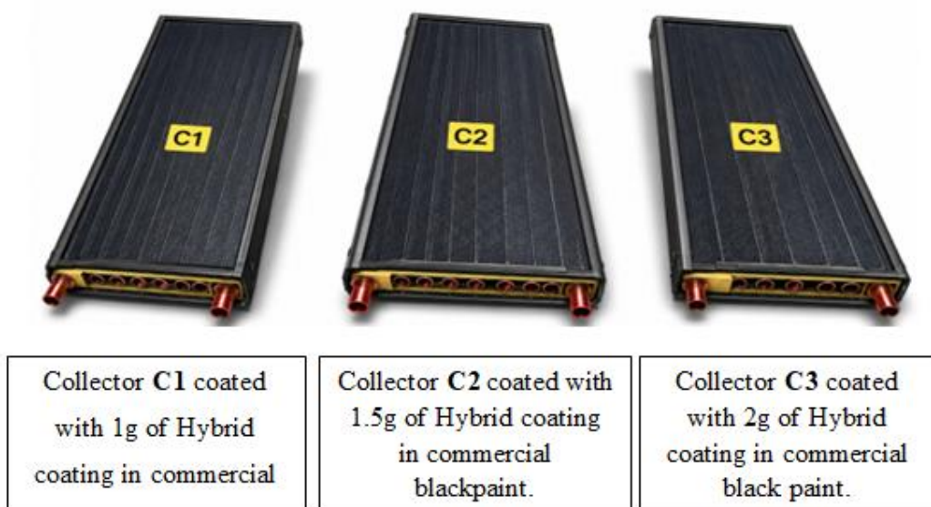
Figure 2. Collectors coated with nano particulars with different ratios
