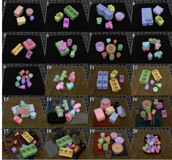
Fig. B4 Visualization of T-LESS scenes. The scenes present up to 18 instances of different objects, with a lot of occlusions and with ambiguous objects. T-LESS is really suited for pose distribution evaluation. (illustration borrowed from [14])
