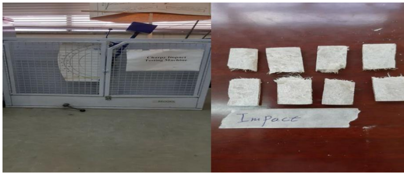
Fig.10: Impact strength tested specimens: (a) Charpy impact testing machine ( b) sample
