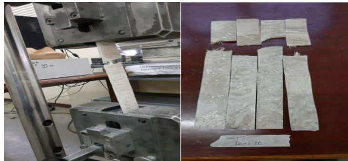
Fig.7: Tensile tested sample ;( a) Tensile testing machine (b) The sample after taste
