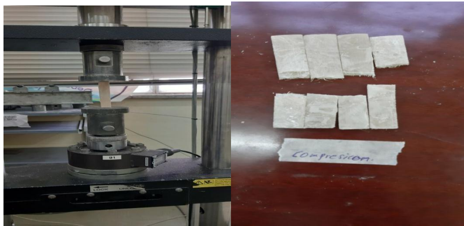
Fig.11: Compression strength tested sample: (a) Compression tested sample (b) The sample while being tested
