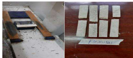
Fig.9: Flexural strength tested specimens: (a) Flexural testing machine and the sample (b)
