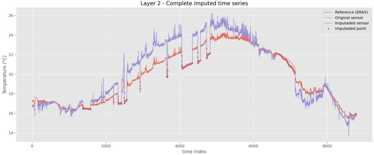
Fig. 8 Time series data of the soil thermal profile in the intermediate layer: sensor data and reference series.
