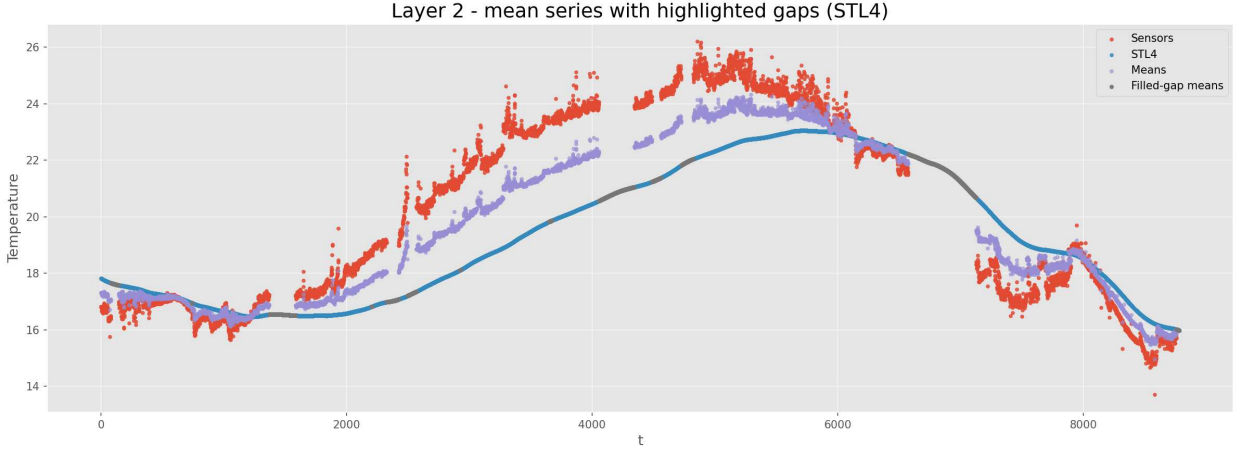
Fig. 6 Time series data of the soil thermal profile in the deep layer: sensor data and reference series.
