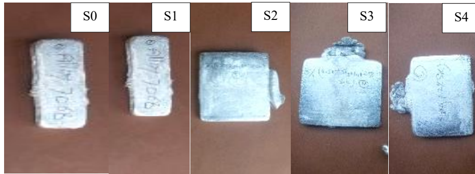
Fig. 4 Al7068 Casted Sample and its Composites
