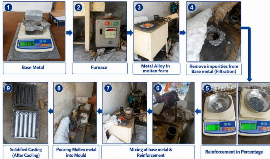
Fig. 3 Sample Preparation Process with SiC & Si 3 N 4
