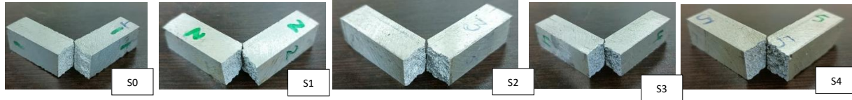
Fig. 9 Specimen after Charpy Test before shot peening
