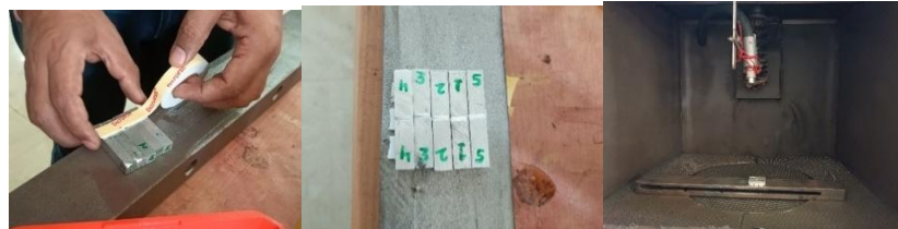
Fig. 12 Specimen's placed in the Shot Blasting Chamber
