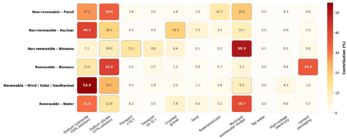
Fig. 6 Cumulative Energy Demand (CED) heat map showing the distribution of fossil, nuclear, and renewable energy (hydropower, wind, geothermal, and solar) for the production of 1 m 3 of geopolymer concrete
