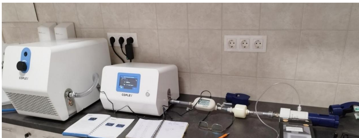
Figure 2. Experimental setup for the demonstration of flow resistance equivalence
