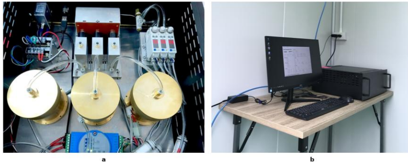
Fig. 2 Photographs of the prototype in the PM10/PM2.5/PM1.0 configuration (enclosure 48.62 \times 22.15 \times 43 cm): a internal layout, showing the three Faraday-cup assemblies with their impaction stages, the high-voltage supply, and the data-acquisition board; b the instrument installed in a monitoring shelter, with the conditioned sample line entering from the ceiling and the control and display computer alongside
