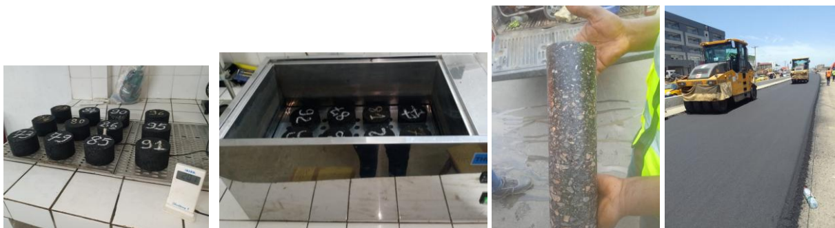
Fig. 10. Cylindrical specimens compacted in 100-mm diameter molds for ITSR test
