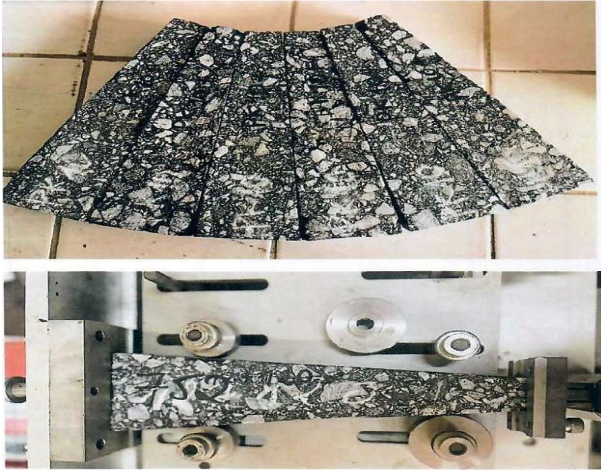
Fig. 15. Trapezoidal specimens sawn from the slabs for fatigue testing
