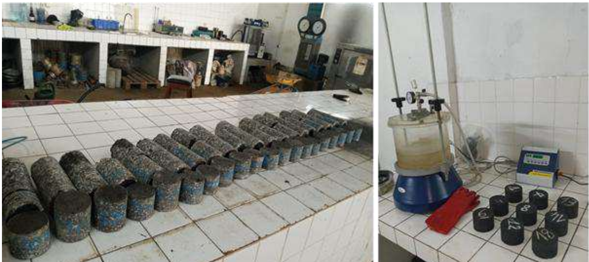
Fig. 14. Cylindrical cores extracted from the slabs and tested using the indirect tensile stiffness modulus method
