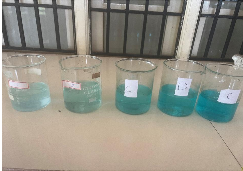
Fig. 3.a. different concentrations of copper sulphate solution
