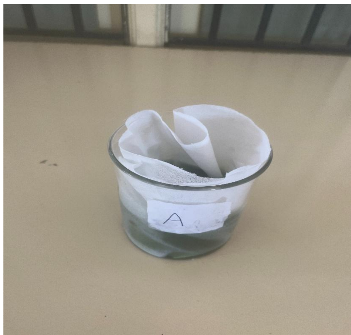
Fig. 2. (b) cellulose matrix immersed longitudinally in the concentrated plant extract
