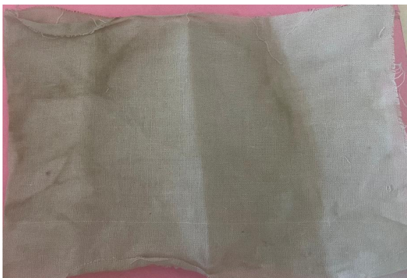
Fig. 3. (c) dried cellulose-supported copper nanocomposite turned to olive green colouration.
