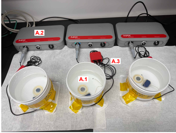
Fig. 3: Image of three (A.1) ANI devices connected to (A.2) MAXbox interfaces for controllers using (A.3) magnetically attached MAXCoil-S for stimulation stability testing or TAA voltage matrix measurements. The 300 mL polypropylene containers are shown with sealing lids removed to reveal the ANI devices immersed in 150 mL 1\times PBS.
