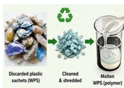
Fig. 1. Converting plastic waste to useful anticorrosion material
