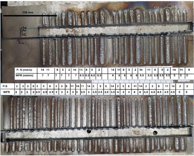
Supplementary Fig. 5 Single bead deposition at 22V
