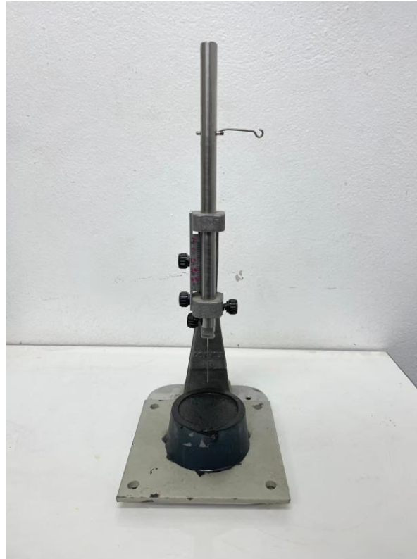
Fig. 5 Penetration-resistance setup used to determine initial and final setting times
