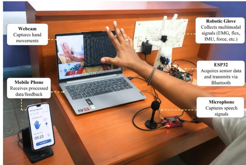
Figure 2. Multimodal Data Acquisition Setup for Parkinson's Disease Rehabilitation
