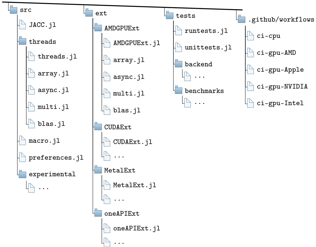
Fig. 12: JACC extensible internal code structure, which reuses Julia’s package structure and includes optional package dependencies ( ext ) for GPU backends.
