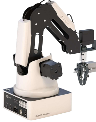
Fig. 1 Perspective view of the 4-DOF Dobot Magician robotic manipulator equipped with a pneumatic gripper end-effector.
