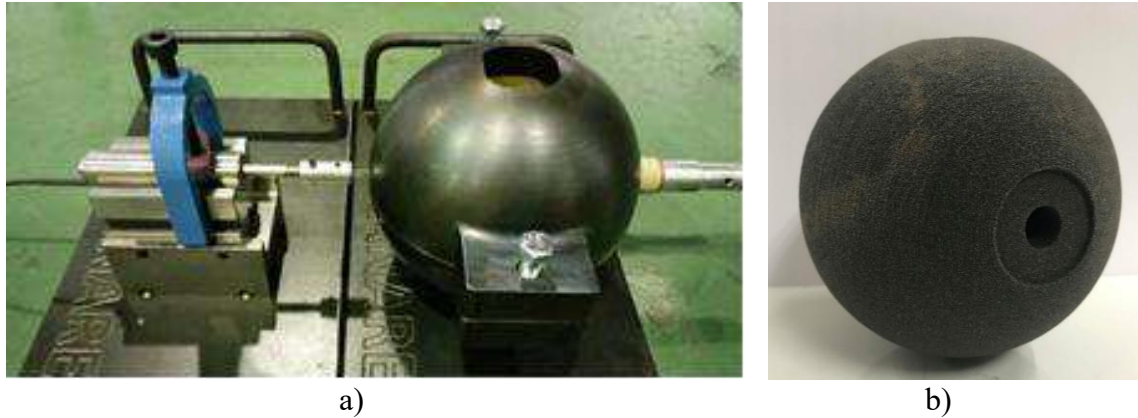
Figure 2 The TA-LDA apparatus; a) the setup (without the lid); b) the additive manufactured sand mold showing the seamless design and the socket for the thermocouple setting.
