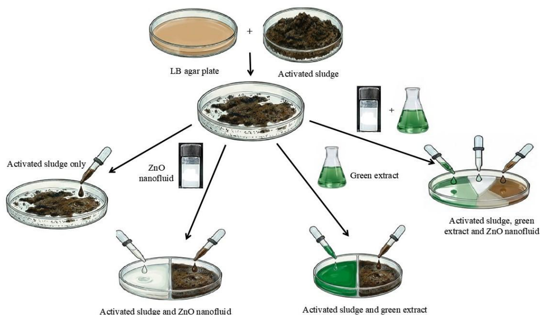
Fig. 4A Schematic representation of microbial enrichment using activated sludge in the presence of ZnO nanofluid and plant-derived phytochemicals prior to wastewater treatment.
