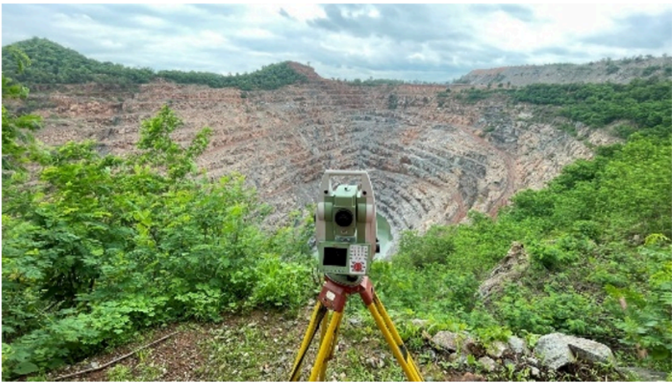
Figure 3 Total station-based surveying method of monitoring to measure slope movement (Wyllie and Mah 2004)
