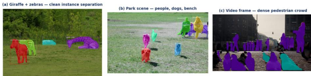
Figure 10. Mask R-CNN qualitative results on COCO-domain imagery and video (ResNet-101 backbone).
