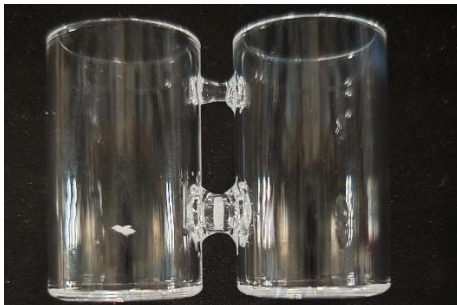
147 Figure 3 Digital photograph of the H-type electrolytic cell assembly. Two cylindrical 148 quartz compartments (35 mm outer diameter, 60 mm high) are connected by a narrow 149 quartz tube (10 mm outer diameter) containing a 2 mm thick glass frit.
