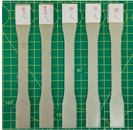
Fig. 4 HDPE-HPS Blends Specimen Following the ASTM D638 Type-I
