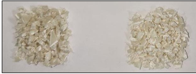
Fig. 2 Sample Image of Crushed Resin of HDPE-HPS Blends
