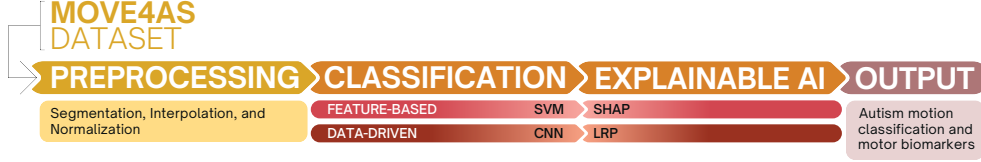
Fig. 1: Overview of the proposed interpretable classification pipeline. Using the motion capture data from the Move4AS dataset [17], the raw data first undergoes preprocessing to ensure signal consistency. The architecture then splits into two parallel streams for analysis: a feature-based classification explained via SHAP, and a data-driven classification interpreted using LRP.
