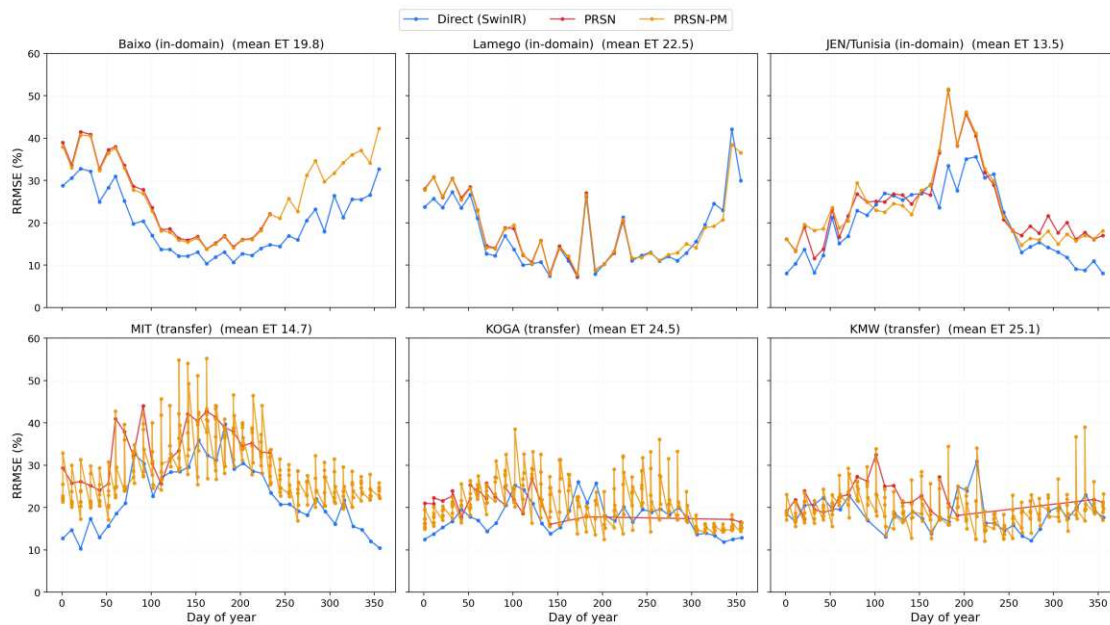
Figure 4. Per-dekad RRMSE (%) versus day-of-year by site, for the direct SwinIR and the two physics models. Error peaks in the high-ET growing season; the direct model lies below both physics models in nearly every dekad.
