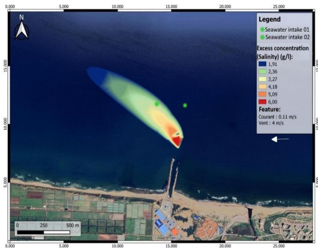
Fig. 10 Brine discharge plume of the Corso SDEM under intermediate velocity conditions ( V = 4 m/s and U = 0.11 m/s)
