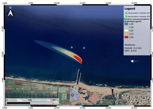
Fig. 7 Brine discharge plume from the Corso seawater desalination plant under favorable conditions ( V = 8 m/s and U = 0.2 m/s)
