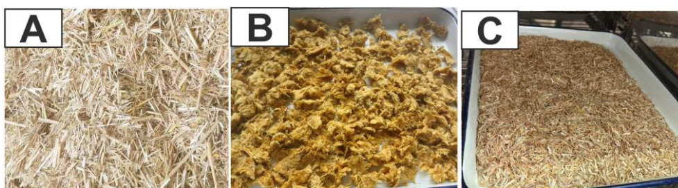
Fig.3. Appearance of wheat straw subjected to different surface treatments: (A) unmodified wheat straw, (B) alkali-treated wheat straw, and (C) silane-modified wheat straw.
