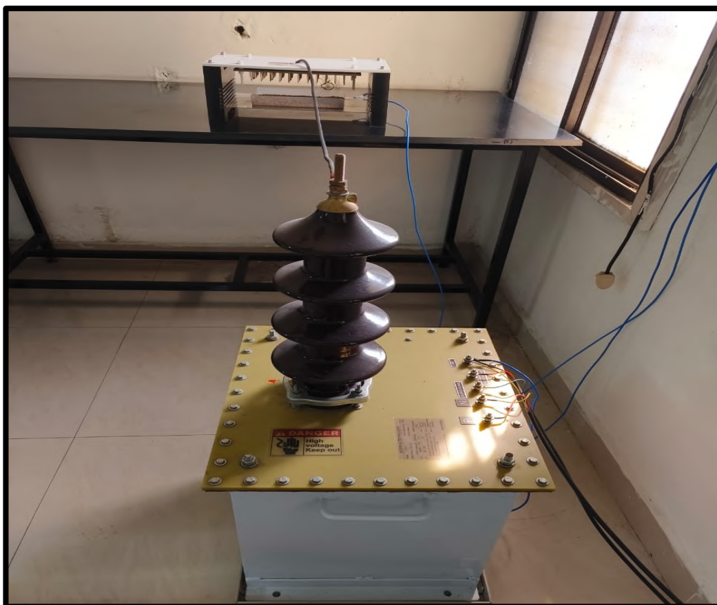
Plate 3.1 Non-thermal plasma device used for treating paddy seed
