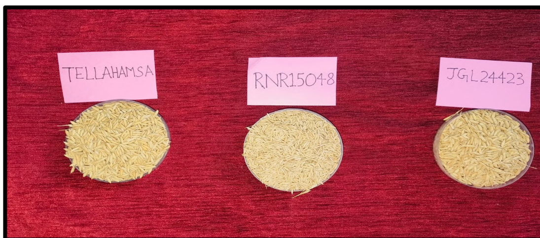
Plate 3.2 Three varieties of paddy treated with cold plasma (20kV for 15 minutes) used for field studies
