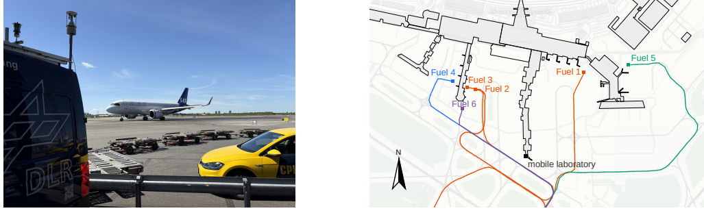
Fig. 1: Measurement setup on the apron at Copenhagen Airport. Photograph (left) showing the mobile laboratory positioned at aircraft stand C39, with the sampling inlet visible on top of the van, and an A320-200neo aircraft taxiing on the adjacent taxiway. Map (right) showing the location of the mobile laboratory on the apron, the taxi routes of aircraft associated with the six selected fuel samples, and terminal buildings (black outlines).
