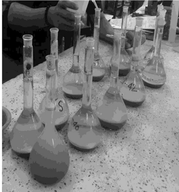
Fig. 4 Representative volumetric-flask testing during index-property characterization of the mixture states
