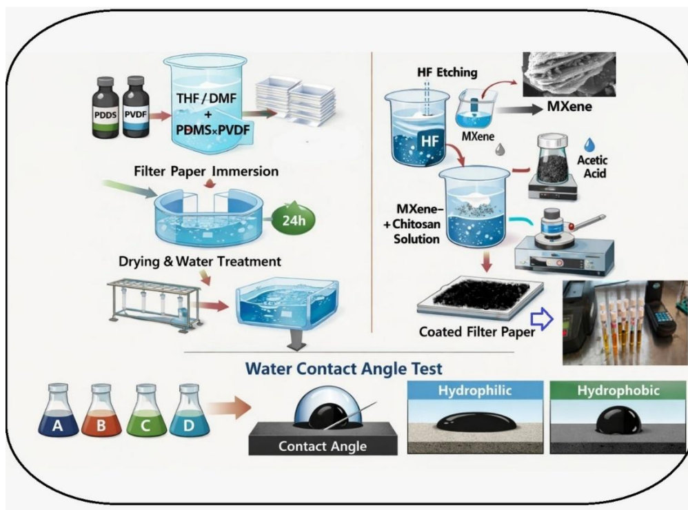
Fig. 2 schematic image of preparation processes of modified filter paper
