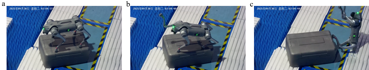
Figure S1: Embodied intelligent robot in a , the initial power-on state, b , the normal operational state, and c , the inoperable state following HPM radiation.
