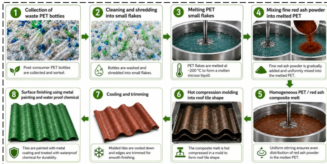
Fig. 3: Schematic diagram of developing eco efficient roof tile from a mixture of waste PET and fine red ash powder.
